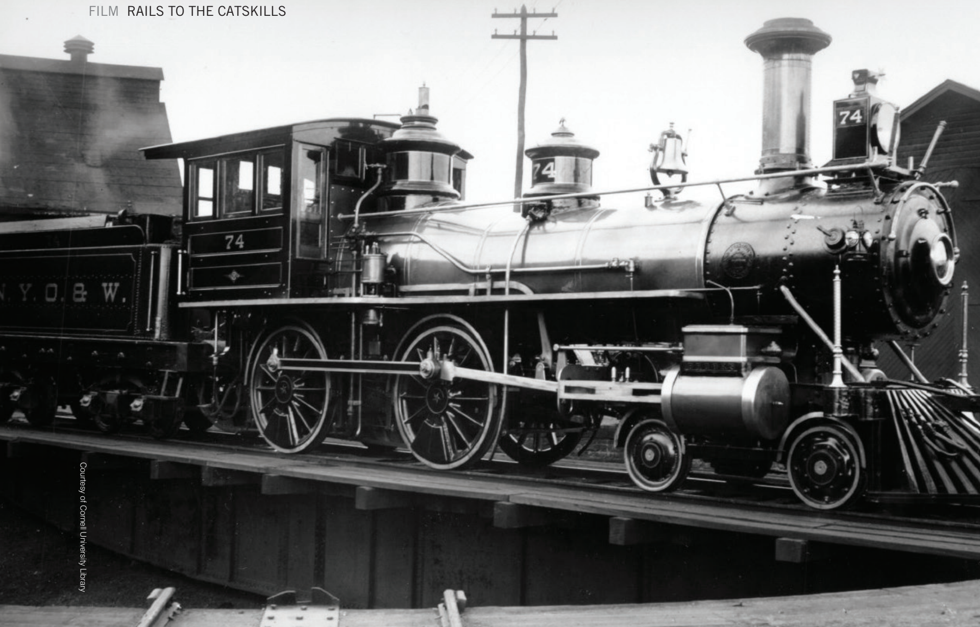
A "Mother Hubbard," or center-cab steam locomotive from the New York, Ontario & Western Railway.
